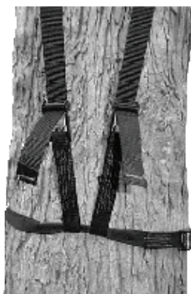
Figure 31 Stabilizer Straps Installed
