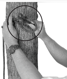
Figure C Slip Knot End Through Loop
