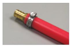
4. Pressure test the PEX tubing and inspect before burying or normal use. If there are any signs of leaks, repeat the total procedure.
