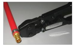
3. Place PEX pinch clamp nub between tool jaws and ratchet the clamp until the PEX Pinch Clamp Tool auto-releases. This action will assure that the PEX pinch clamp is fully engaged.
