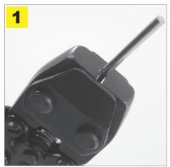
1. Insert the Calibration Bar into the tool as shown. Ratchet the Pinch Tool to the closed position (tool jaws should be biting into the bar).
