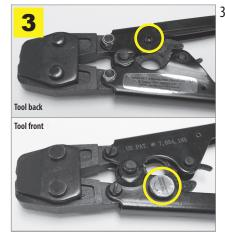
3. To adjust the jaw gap, turn the Pinch Tool on its back and locate the locking screw. Use a standard screwdriver to loosen the locking screw. Turn the tool over and locate the adjustment dial. Turn the adjustment dial right or left as needed to change the size of the jaw gap. When adjustment is complete, tighten the locking screw.
